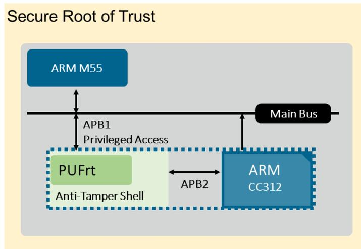
Figure 4. Extend ARM CC312 secure boundary with PUFrt
