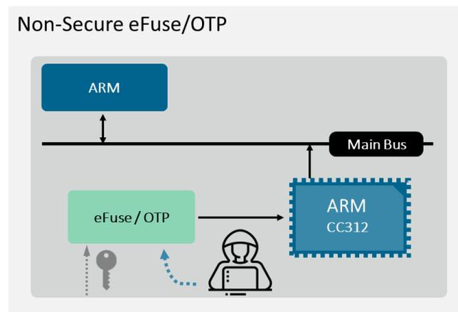
Figure 2. Non-Secure Root of Trust
